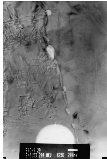
Fig. 9 The pores in the boron carbide coating
